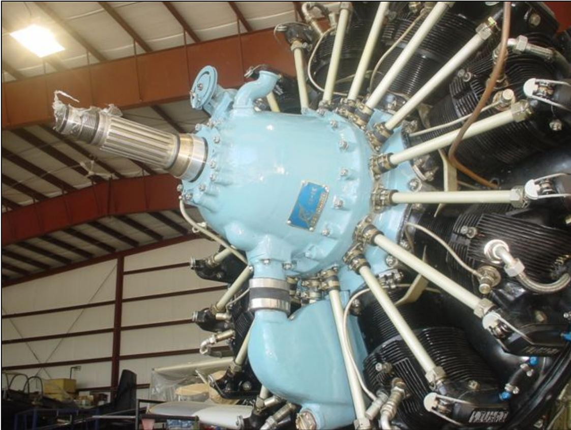
The last and most problematic challenge was remounting the shaft and reduction gearbox into the dome. The shaft journals have metal sealing rings, which are very similar to automobile piston rings. The problem is their need to be compressed while being inserted into the sleeve. As you move the two together, the space available for your hands quickly disappears because the reduction gearbox is very wide and bolts to the backside of the
